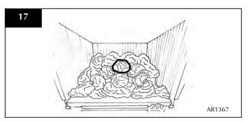
• Place the last two small coals to the left and right-hand side of the bed in the two spaces, Diagram 18.
